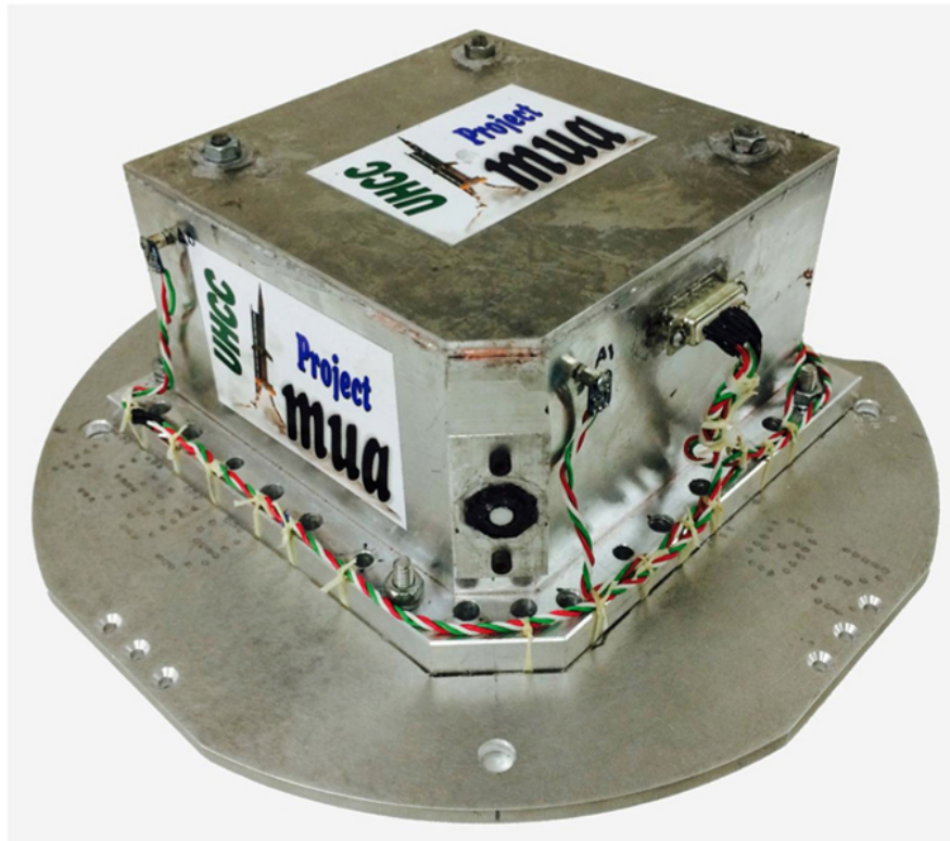
Fig. 2. Payload’s mechanical housing consisting of 6061 aluminum
